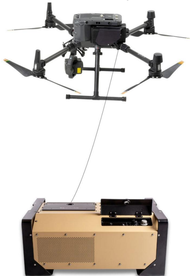
Figure 4. Safe-T2 and DJI M350 drone systems
