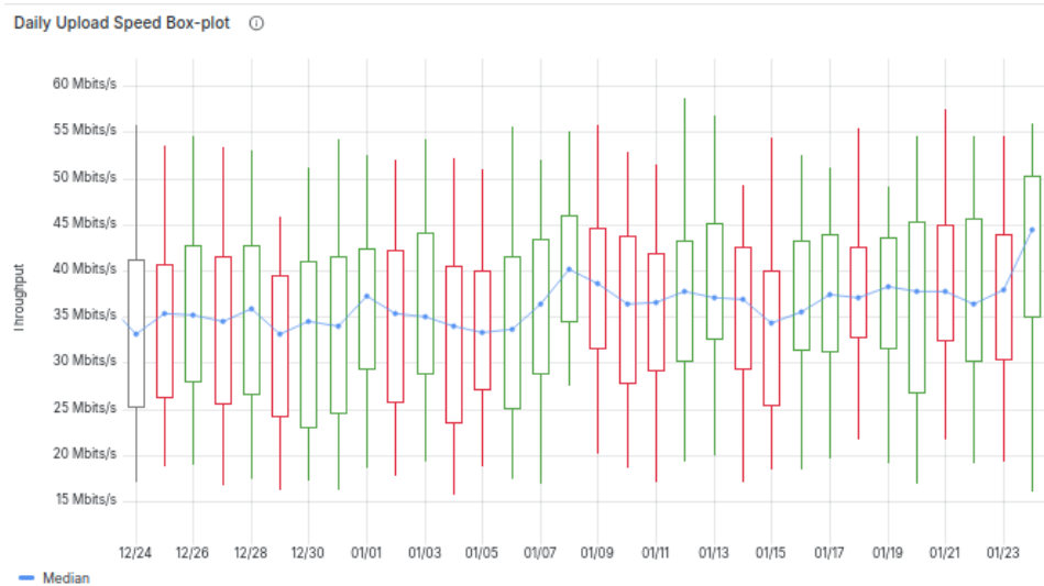
Figure 19. Daily (from the 24th of December until the 23rd of January) Uplink speeds of the Starlink system in Mbit/s.
