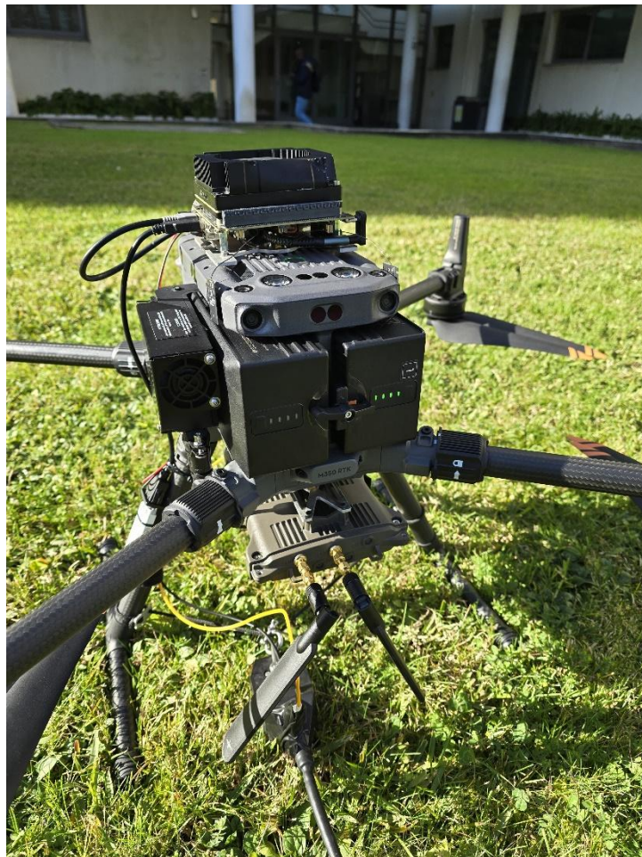
Figure 34. Tethered Drone Air Module connection to batteries and tether cable.
