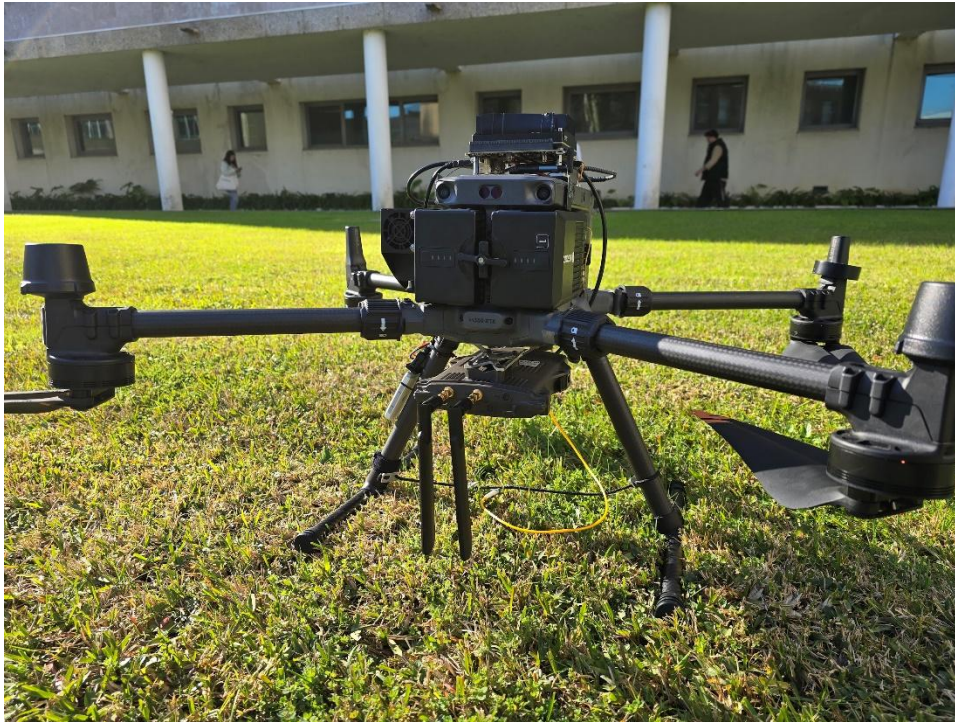
Figure 5. DJI M350 customized with Jetson Orin.
