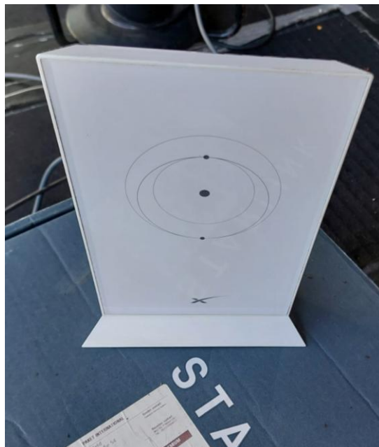
Figure 10. Modem Router and Gigabit Ethernet adapter of the Starlink system.
