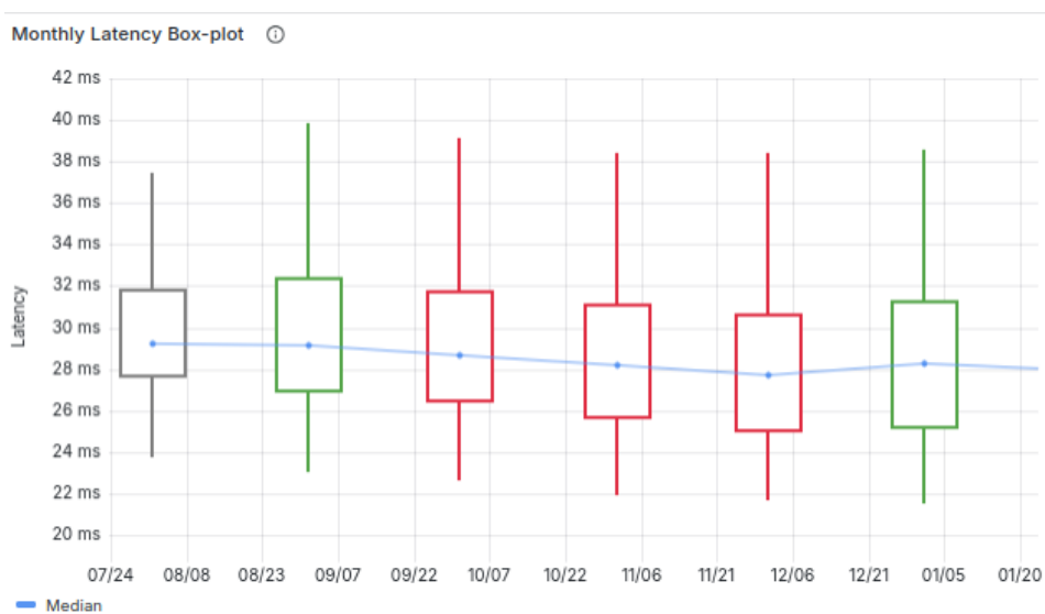
Figure 14. Monthly (from August 2024 until January 2025) Latency (RTT) of the Starlink system in milliseconds.
